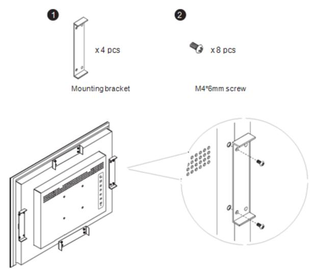
\*\* Remarks: Bracket mounting set is already installed on the back of the LCD panel.
